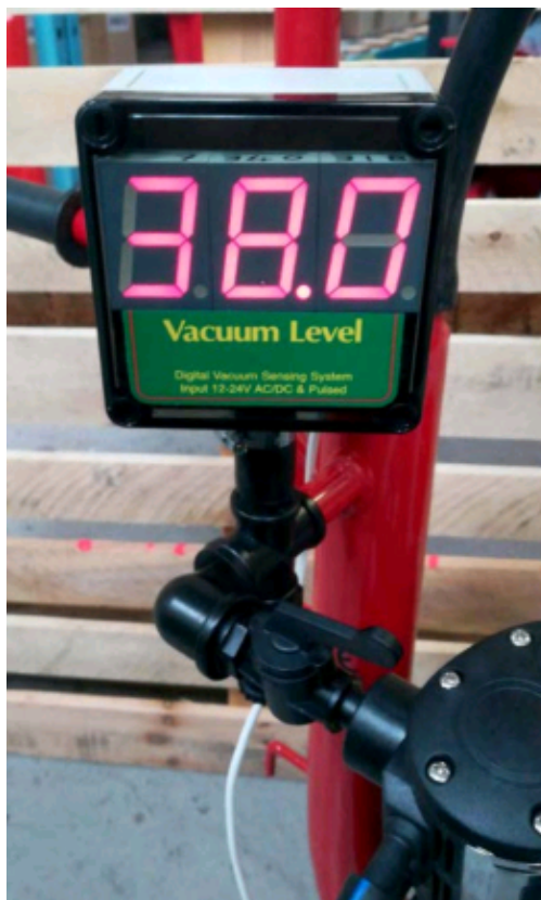
Digital display: an easy-to-read gauge is key to accurately monitoring vacuum levels
